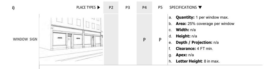
Window Signs shall not interfere with the primary function of windows, that is to enable passersby and public safety personnel to see through windows into Premises and view product displays.
