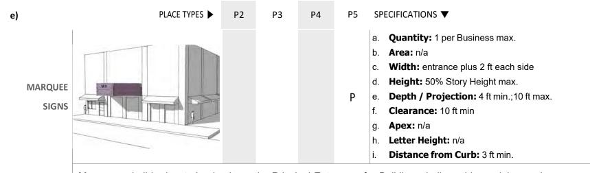
Marquees shall be located only above the Principal Entrance of a Building, shall provide a minimum clearance DESCRIPTION of 10 feet, and may Encroach the Public Frontage to within 2 feet of the Curb. Message Boards shall be permitted as part of Marquees.
