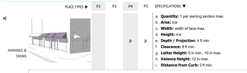
Awning Signage shall be limited to no more than 70% of the Valance of the awning or the vertical portion of a dome awning. The Height of the Valance shall not exceed 12 inches. For a flat roof awning, Awning Signage can extend 12 inches above the top of the awning. Awning Signs shall contain only the Business name, Logo, and/or Street address.
