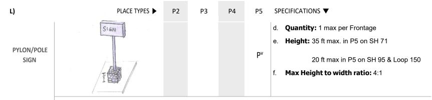
A Sign permanently affixed to the ground at its base by a single- or double-poles, that are enclosed by a base of natural stone, DESCRIPTION stucco, brick, or wood and not mounted to a part of a Building. Only allowed in State Highway 71 & SH 95
